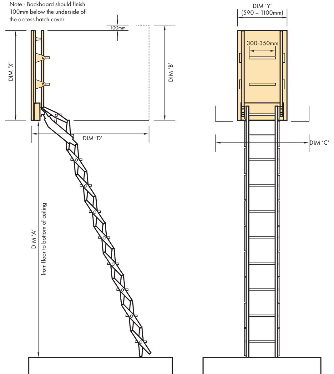
When the BL-Z is ordered with a Backboard, the BL-Z will be delivered fitted to the backboard.
